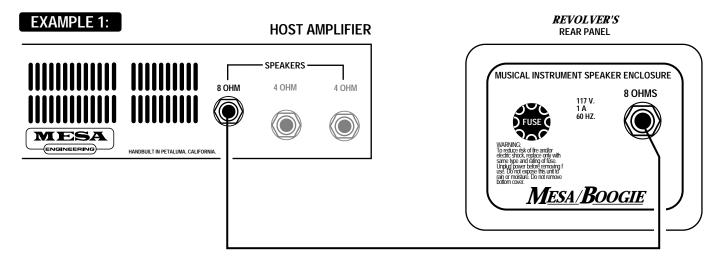
Example 1 is the simplest Hook-Up option for the **REVOLVER** and yields a much deeper effect than when it's used simultaneously with a stationary speaker cabinet.
